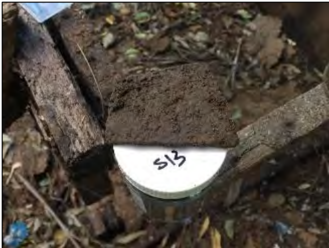
Plate 29 – Fragment of ACM identified in fill at the rear of the truck shed at sample location S13.
