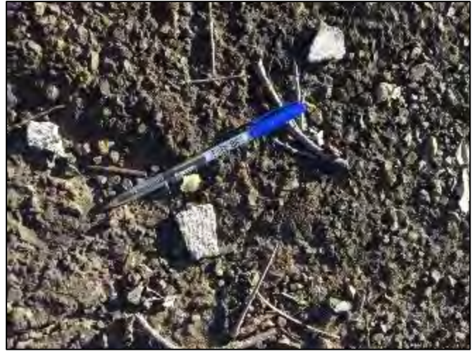
Plate 20 – ACM fragments on asphalt north of the shed.
