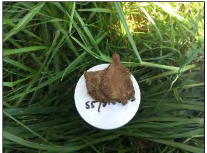
Plate 40 – Fragments of ACM in shallow soils at location S5.
