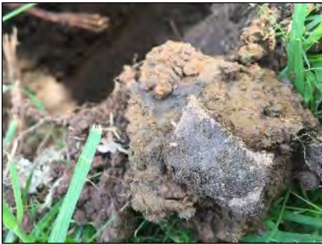
Plate 33 – Fragment of ACM identified in fill soils associated with the tennis court.
