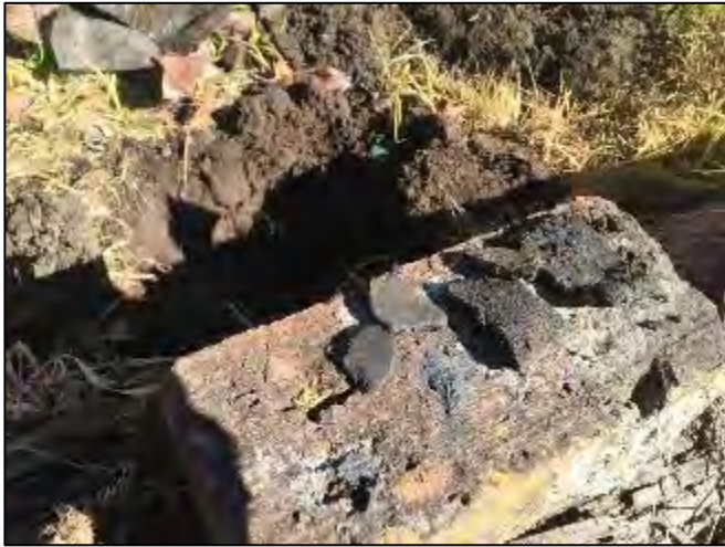
Plate 7 – Fragments of ACM encountered in surface soils at S19 adjacent to the granny flat.
