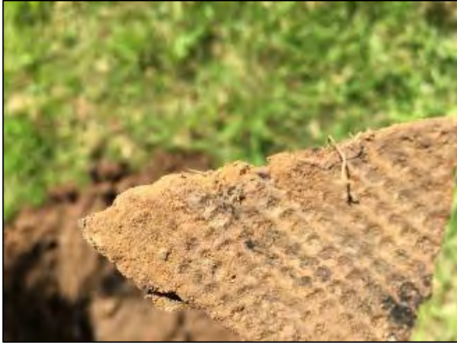
Plate 31 – Fragment of ACM identified in S16 associated with fill near the tennis court.
