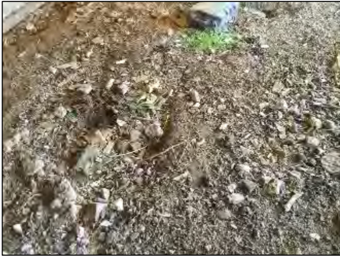
Plate 43 – Fragments of ACM scattered within and surrounding the southernmost shed at sample location SS1.
