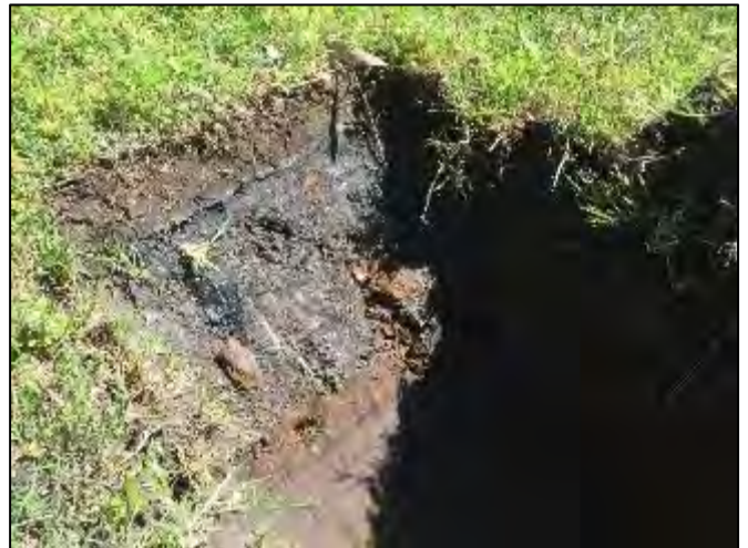
Plate 30 – Typical soil profile in the central portion of the site showing coal wash fill.
